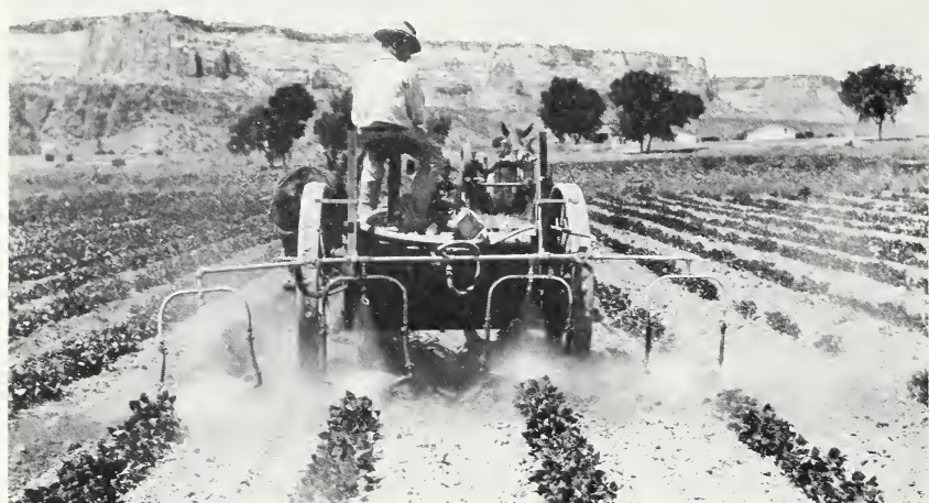
FIGURE 2.—Power sprayer used in experiments on Mexican bean beetle control. Power equipment is essential for obtaining the 150 or more pounds' pressure necessary for effective control.
